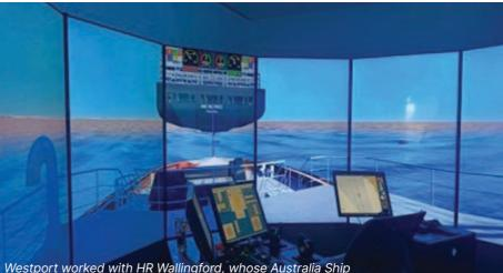
Simulation Centre is located in Fremantle, to test navigation to, and berthing at Westport under dozens of different weather conditions and emergency scenarios.
