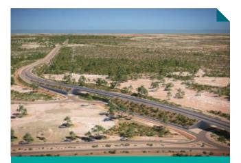
The early road concept for the freight corridor between Clementi Road in Mandogalup and Tonkin Highway in Oakford includes both four and six lanes with a concrete median, and proposed bridges, interchanges and roundabout access at key intersections to provide uninterrupted east-west movement for freight vehicles and enhanced safety for local road users.
